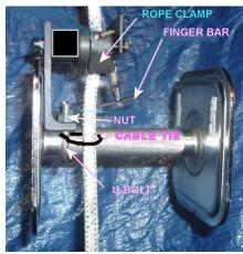
The picture on the left shows the Free-Spotter installed on the dumbbell handle. The *u-bolt* and nuts are used to hold the it in place.
