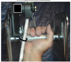
The rope clamps are opened (so the ropes can run free) by gripping the finger bar between two fingers and closing the grip. The user should experiment to find the most comfortable finger combination to use.
